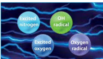
The electrons collide and combine with nitrogen and oxygen in the air to form four kinds of elements.
