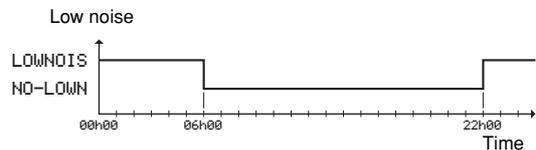
2. Through a field installed low noise mode switch. In this case the low noise mode activation is depending on a changeable digital input: LOW NOISE MODE: CH.DI. Refer to "Customization in the service menu", chapter "Setting of the changeable digital inputs and outputs" in the installation manual.
