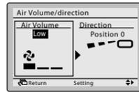
6 With fan speed setting selected, use ▼▲ to select the desired fan speed from Low, Medium, or High.
