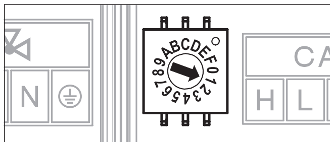
Fig. 9-1 Setting the device ID for the EHS157068 mixer module
