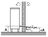
When water is at standstill inside the system, freezing is very likely to happen and damaging the system in the process.
