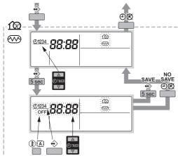
Programming space cooling, quiet mode, or booster heater mode<sup>(1)</sup> is carried out as follows:
