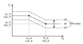
$T_t$  Target water temperature  $T_\Delta$  Ambient (outdoor) temperature
